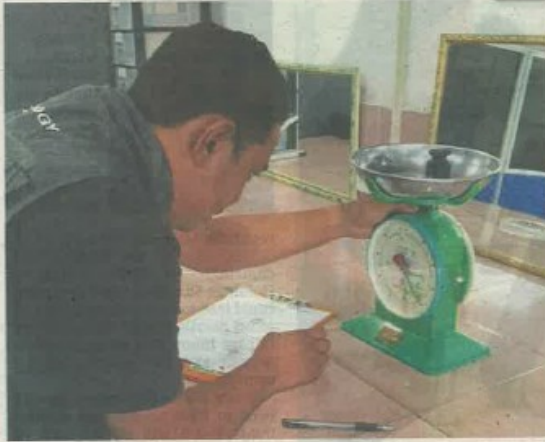
An MCM officer verifying the accuracy of a spring balance.
